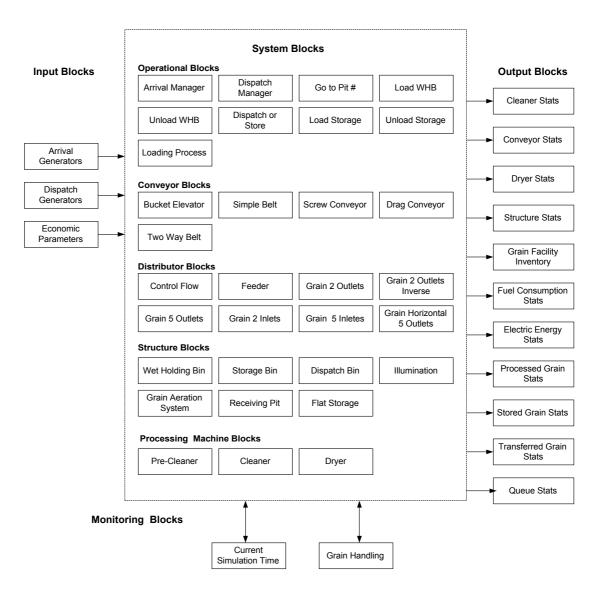
Figure 1- Grain Facility Library schematic representation.
